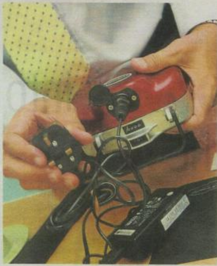
Easy to charge: The lithium-ion battery used in Ezzy Rider's vehicles takes about 30 minutes to an hour to recharge and can last up to 40km on a bicycle.
